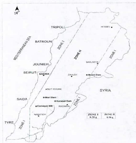
**Figure 2 :** Dams and Conveyors Location with Respect to the Seismicity of Lebanon
